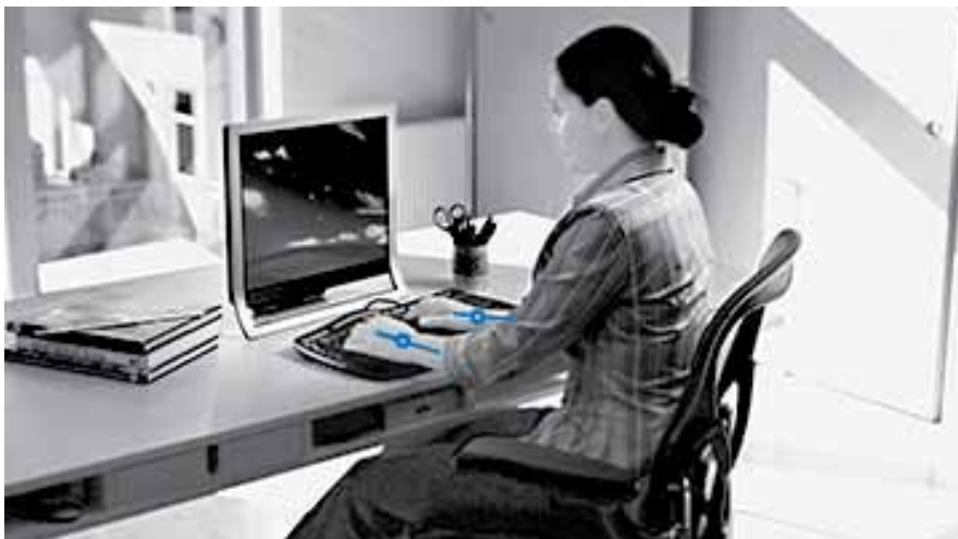
Figure 1. A split keyboard reduces ulnar deviation, twisting of the nerve on the little finger side of the forearm.
