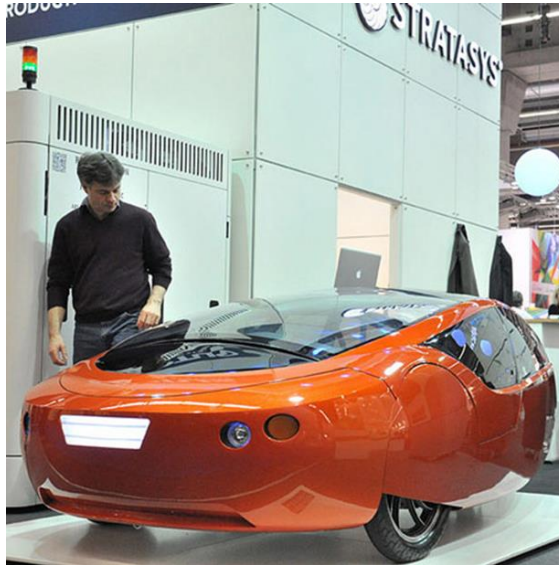
Figure 13: The Urbee First Fully-functional 3D Printed Car
