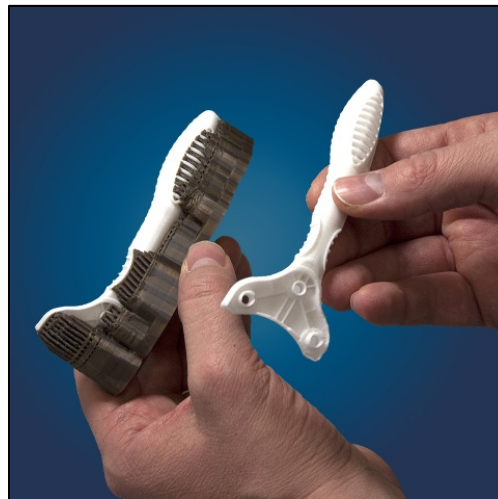
Figure 16: Before and After with Support Material
