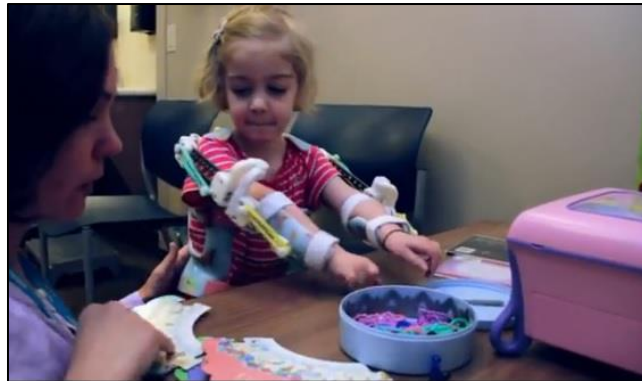
Figure 11: A Child with a Custom 3D Printed Exoskeleton
