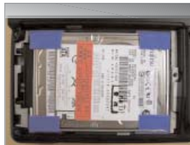
> HDD Protection: a combination of shock-absorbing material and Toshiba's own three-axis motion monitoring system.
